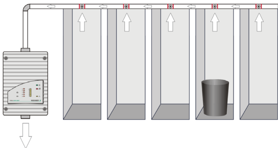
Figure 5: Phase 1 ROOM-IDENT standard operation
