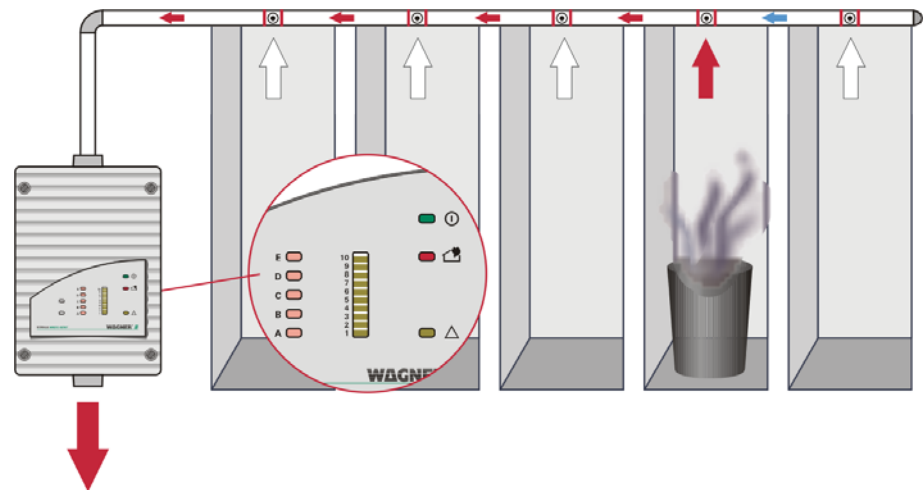
Figure 6: Phase 2 ROOM-IDENT earliest fire detection
