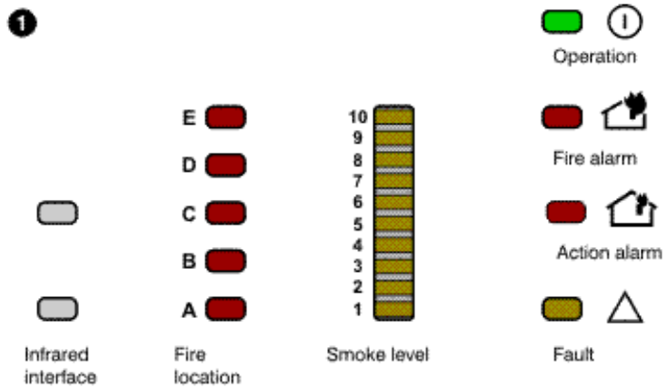
Figure 12: TITANUS MICRO-SENS® display variant with smoke levels and fire location
